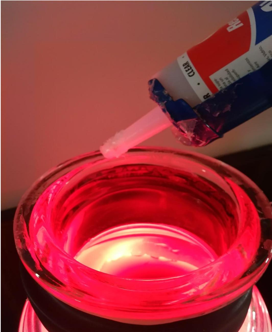
**Remove the Red silicone rubber from the boiling water and pat dry thoroughly. Carefully place it onto the fresh silicone and then put a flat compress on top of it (I used a stack of heavy books)**
